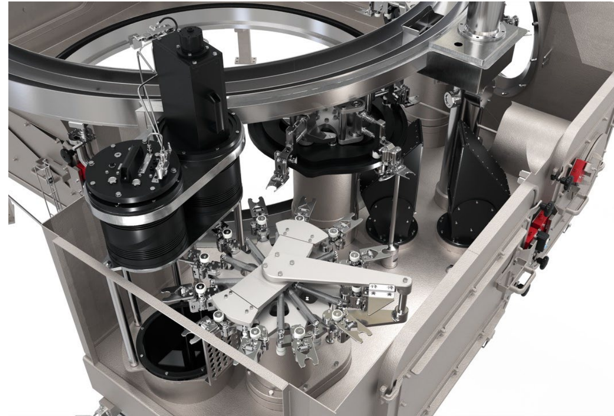
Sealing surfaces inspection in the Contipure AseptBloc
